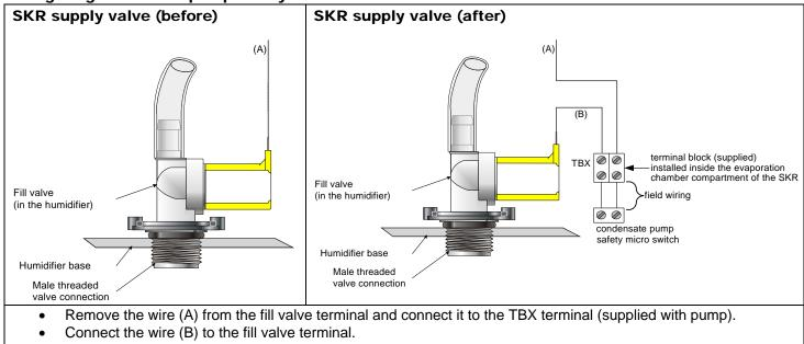
• Make the connections between the TBX terminal and the condensate pump safety switch.
